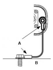
The eyelets must be crimped or soldered at both locations (A) and the method of connection to the vessel's hull is shown at (B).
